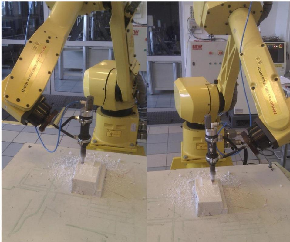
*Fig. 4. Example of machining of workpiece from polystyrene*
