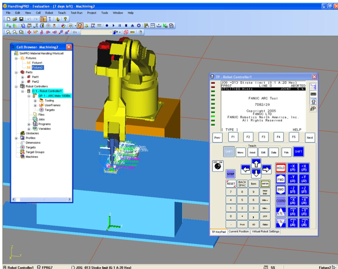
Fig. 1. Virtual model of robotic workcell for machining in RoboGuide
