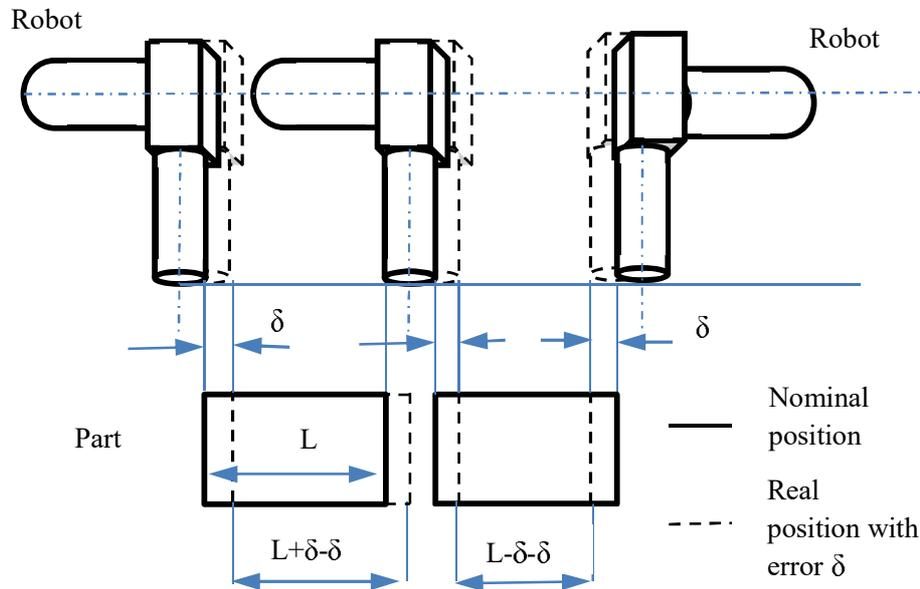
Fig. 3. Robot tool error  $\delta$  and part accuracy
