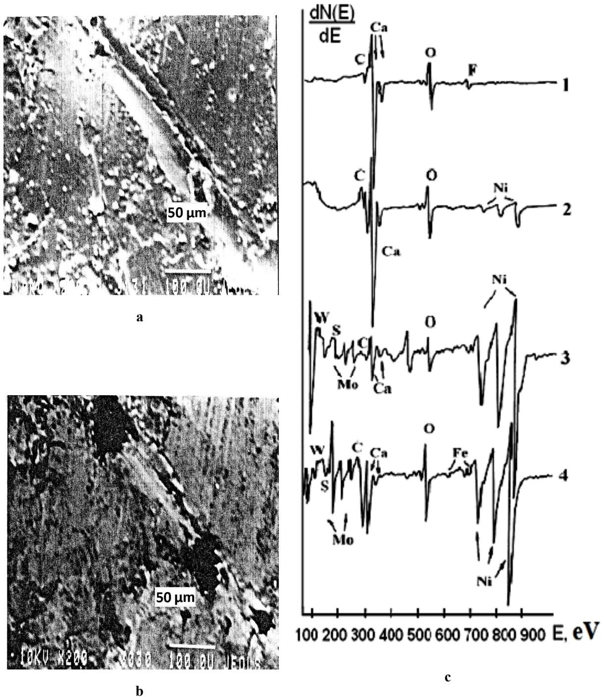
Fig. 6. The friction surface of the material (Ni-Mo-W) +10%CaF<sub>2</sub> after tribological testing at 9 MPa: a - dripping traces and brittle cleavages; b - friction track in a mode of composite contrast; c - Auger spectra (1 - dark field, 2, 3 - brightfields, 4 - wear products)
