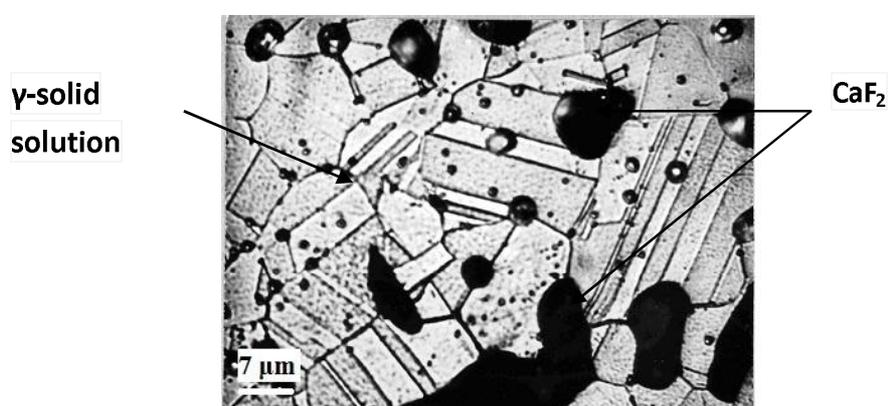
Fig. 1. The structure of material 63Ni + 13.5Mo + 13.5W + 10CaF<sub>2</sub>
