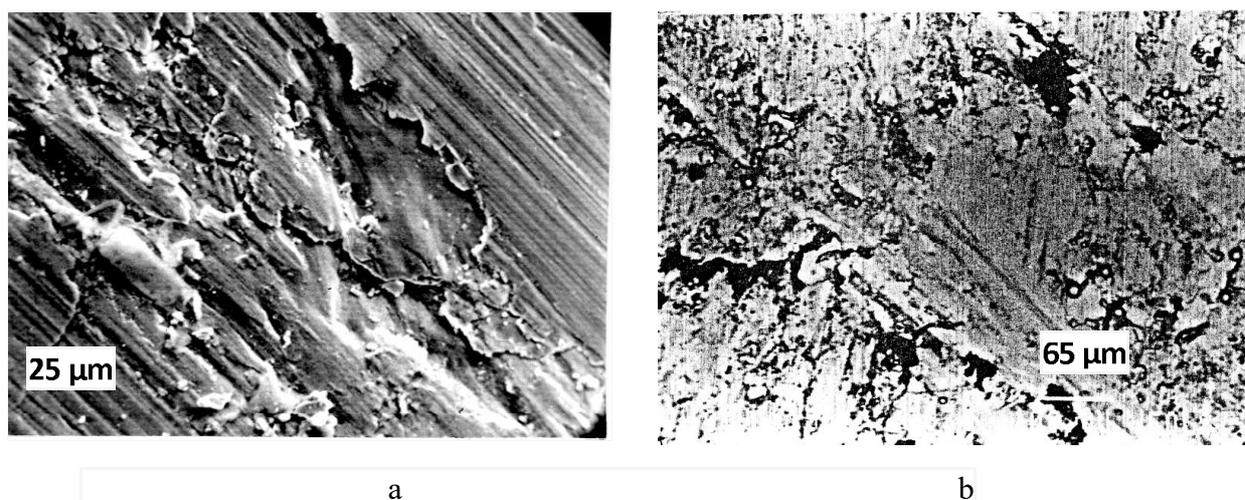
Fig.3. The material (Ni-Mo-W) +10% CaF<sub>2</sub> friction surface's fragments after tribological tests at 7MPa: a - secondary structures' topographic relief; b - image in the Auger electrons
