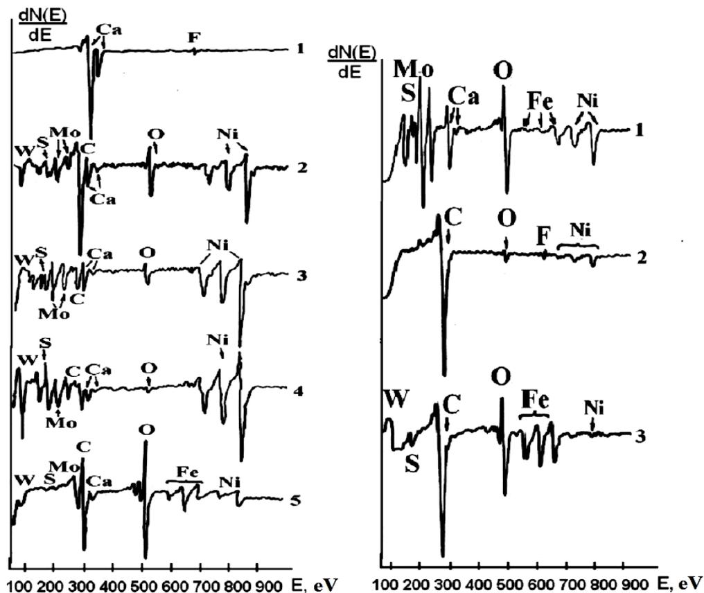
Fig.2. Augerspectrum of the surface layer after the tribological tests at a pressure of 5MPa: a- the material (Ni-Mo-W) +10% CaF<sub>2</sub> (1 - white portions, 2,3 - smooth surface areas, 4,5 - wear products) b - counter face of steel EI961 (1 - smooth light area, 2 - smooth dark zone, 3 - wear products).
