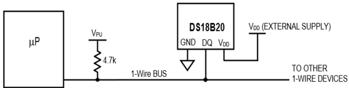
Fig. 1. Diagram of the sensor supply DB20B18 [1].
