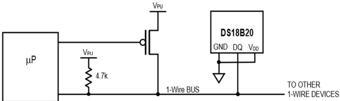
Fig. 2. Scheme of parasitic supply of sensor DB20B18 [1].
