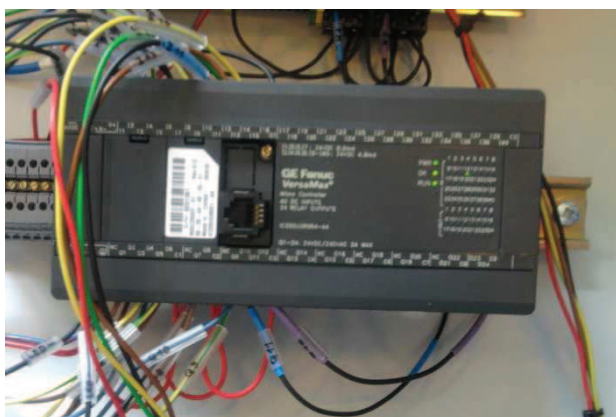
Rys.7. Widok sterownika VersaMax Micro IC200UDR064 Fig.7. The front view of the VersaMax Micro IC200UDR064 controller
