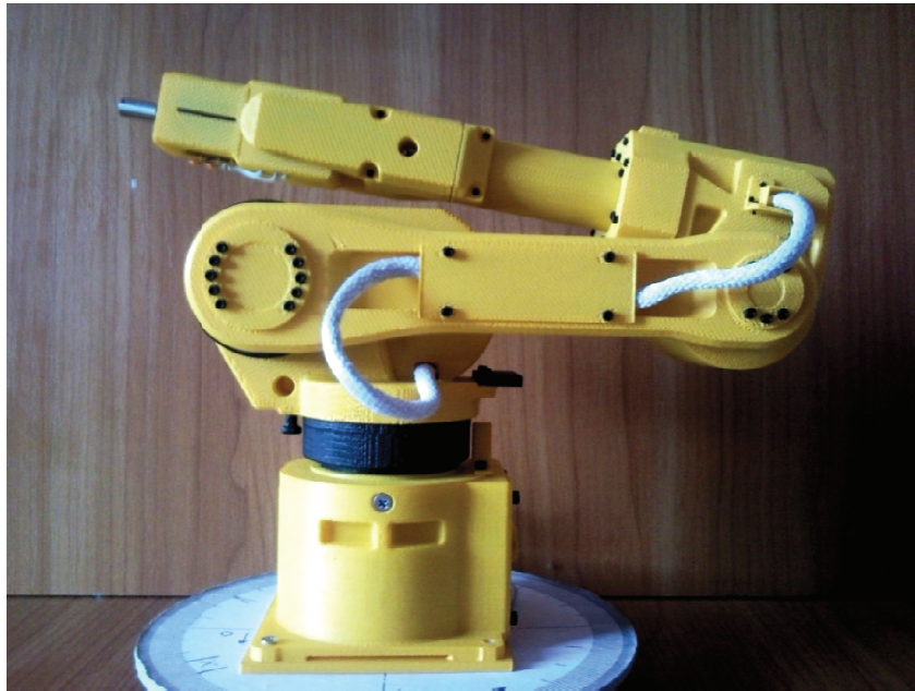
Rys.6. Gotowy model robota FANUC ARCMate 100iB w skali 1:4 Fig.6. Finished robot model FANUC AM100iB in 1:4 scale
