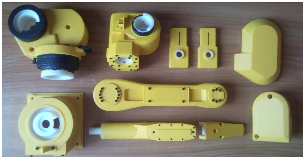
Rys.4. Elementy modelu robota po procesie lakierowania Fig.4. The robot's elements after painting process
