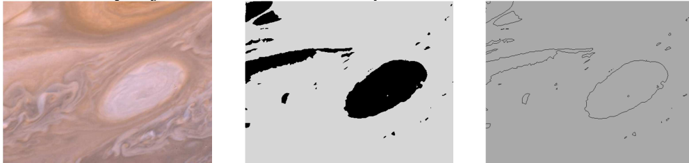
Fig. 3. At the left the fragment of a photo of Jupiter with an atmospheric whirlwind is represented. In the middle the same fragment on one of stages of processing of the image is represented. On the right results after reception of contours, before the beginning of process of recognition are represented. It is easy to notice that using of difficult methods of recognition here is not required and enough to use identification by quantity of points for defect definition.
