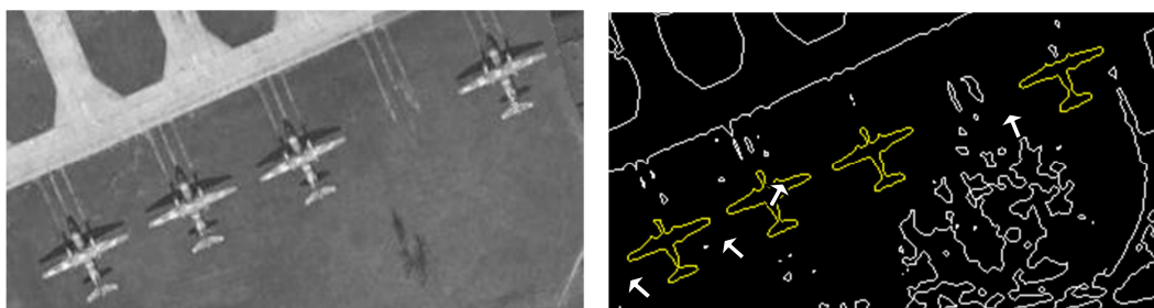
Fig. 6 At the left to show fragment of Balice Airport, Krakow, Poland. From write – this image after processing. The recognized planes noted white arrow.
