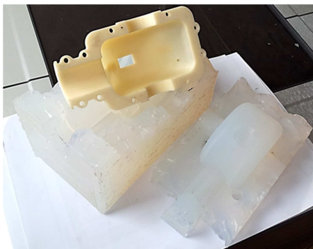
Fig.11. The master model taken out from the silicone form
