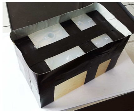
Fig.12. The silicone form read for a casting of a new product
