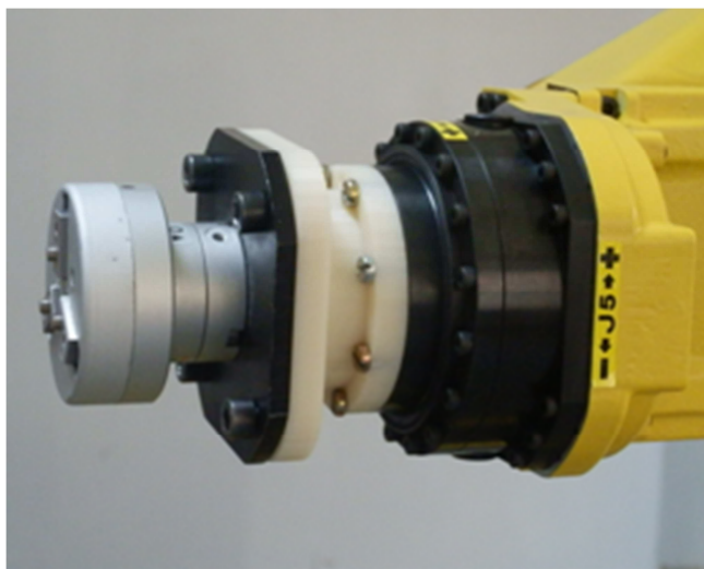
Fig.2. Finished adapter (white) mounted on the robot
