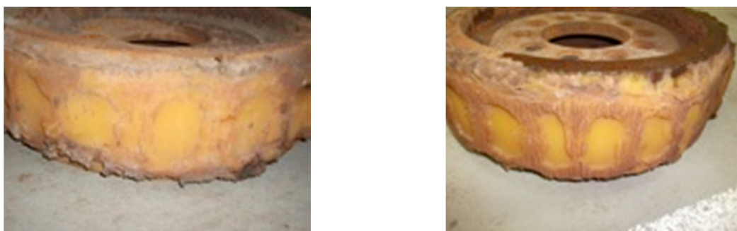
Fig.3. Images of the correctly produced and used drive wheels
