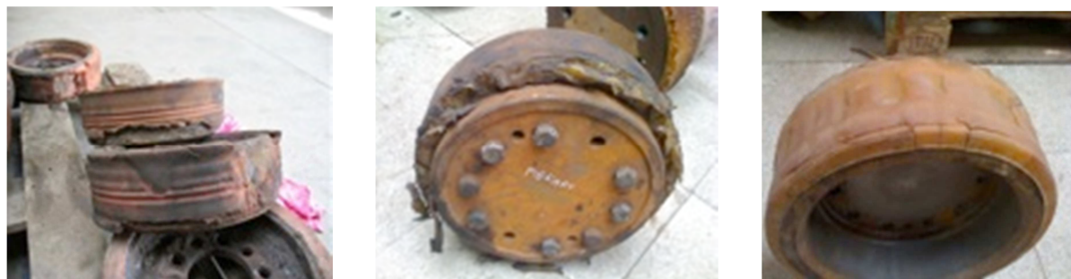
Fig.5. Drive wheel damaged during use
