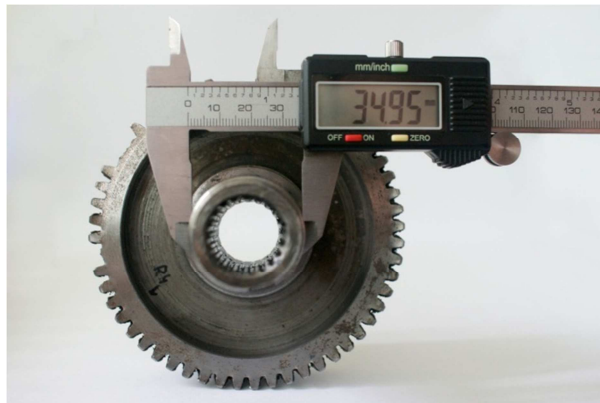
Fig. 2. Measuring external diameter of a roller
