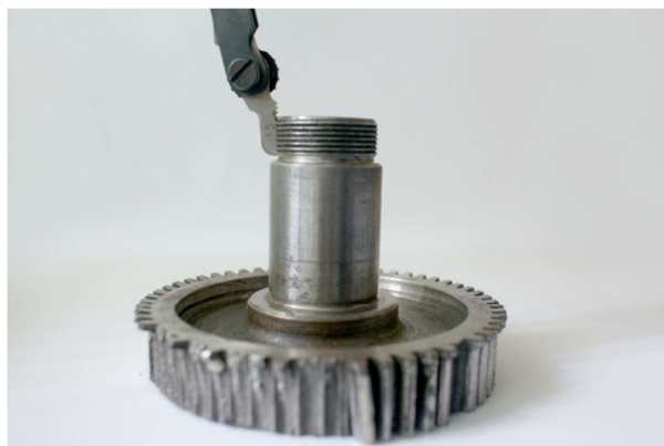
Fig. 3. Identifying the lead of the screw thread
