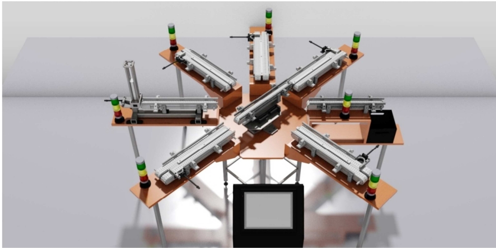
Fig. 4. Visualisation of the discrete manufacturing processes control station
