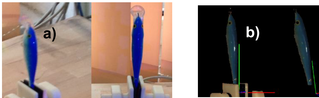
Fig. 5. The scanning process of the wobbler model, a) the wobbler model fixed in the handle, b) the appearance of the wobbler model in 3D Mesh software
