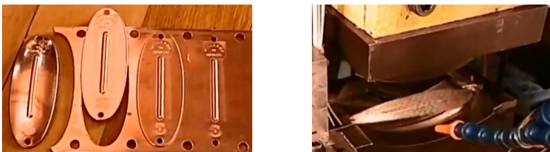
Fig. 3. Stages of the spoon lures manufacturing process [9]
