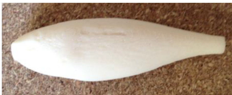
Fig. 7. The wobbler model made with fused deposition modelling on FDM 360 MC machine [10]
