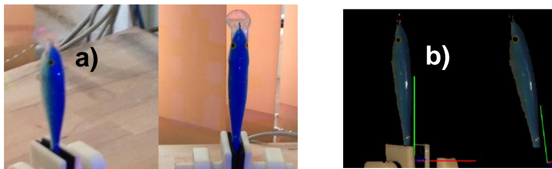
Fig. 5. The scanning process of the wobbler model, a) the wobbler model fixed in the handle, b) the appearance of the wobbler model in 3D Mesh software
