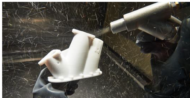
Fig.1. FDM model beat blasting [3]
