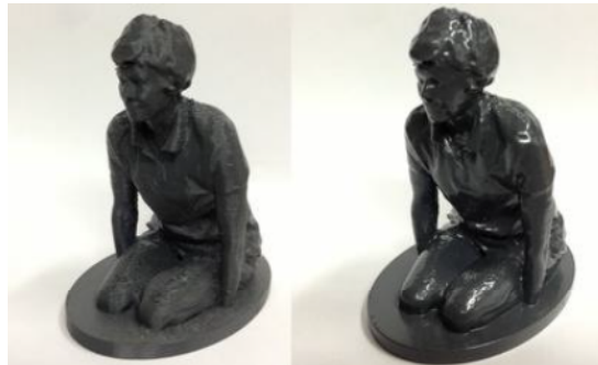
Fig.3. The model smoothed in smoothing station [4]
