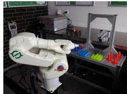
Fig. 1. The K-ROSET 3D simply model and expanded real laboratory station with Kawasaki RS005L robot
