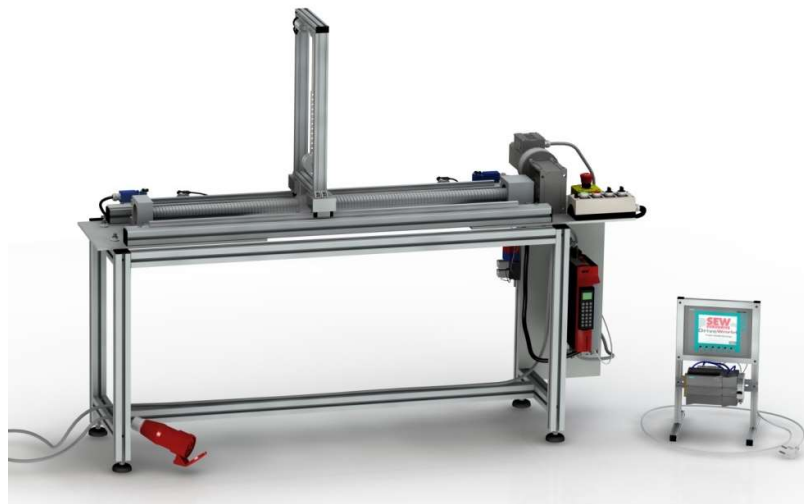
Fig. 1. View of 3D model of the laboratory stand (a mechanical subsystem and control units)
