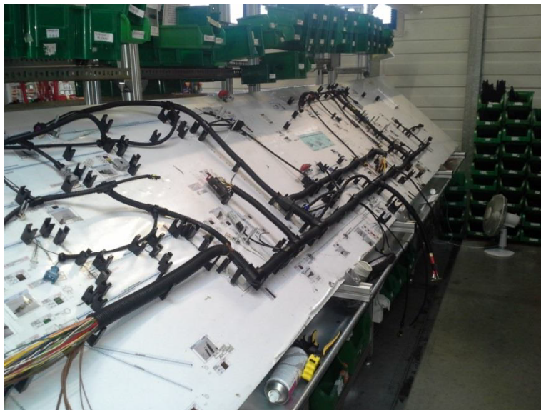
Fig. 4. Assembly table for middle-series and mass production of wire sheaves
