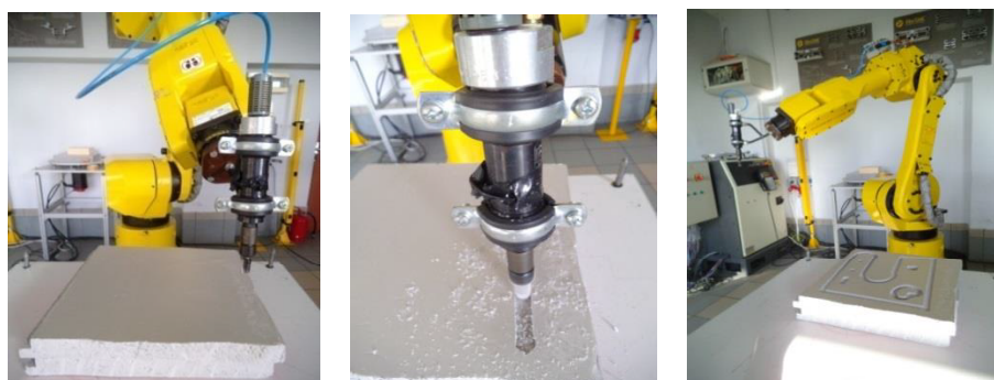
Fig. 1. The rapid prototyping station with Fanuc ArcMate100iB industrial robot
