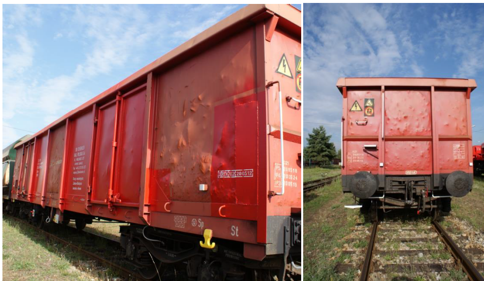
Fig.1. The considered freight wagon and damage of the body shell
