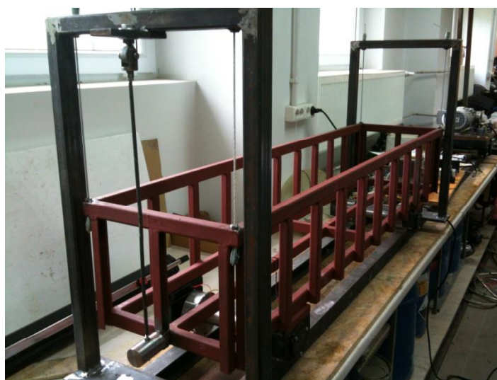
Fig.3. The simplified laboratory model of the supporting structure
