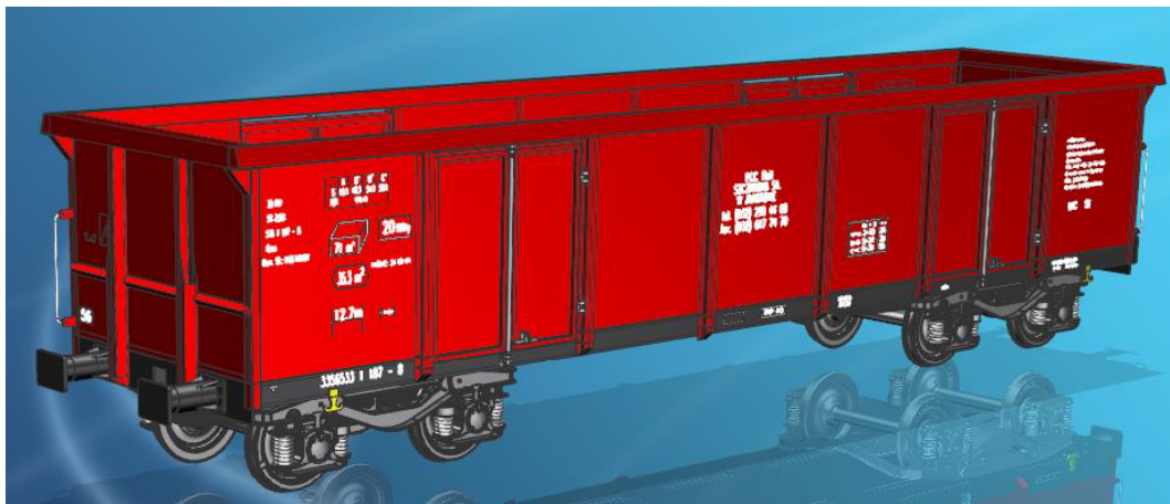
Fig.2. The CAD model of the considered type of freight car
