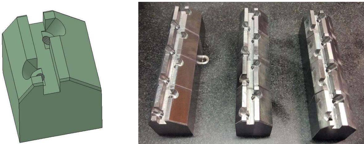
Fig. 5. Model and 3 series of control items: series 1. (left) made only with the help of angular vise; series 2. (middle) produced by peripheral milling method and also with the help of angular vise; series 3. (right) made only with help of designed tilting table.
