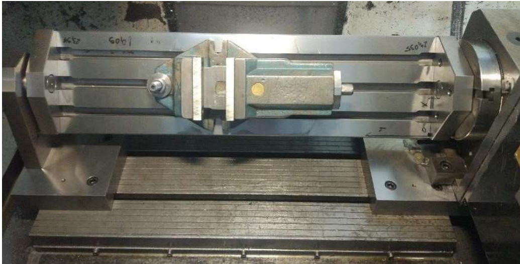
Fig. 4. Ready assembled tilting table in machine with example vise
